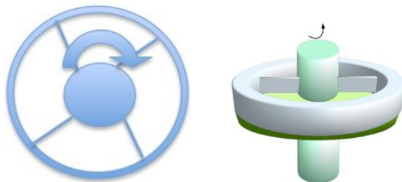
Figure 4: Torsional snap through element with negative incremental torsional rigidity. Left, top view; right, perspective view.
